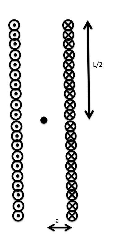
Magnetic field at the center of the solenoid
