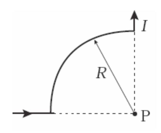
The segment of wire (total length = 6R) is formed into the shape shown and carries a current I. What is the magnitude of the resulting magnetic field at the point P?
